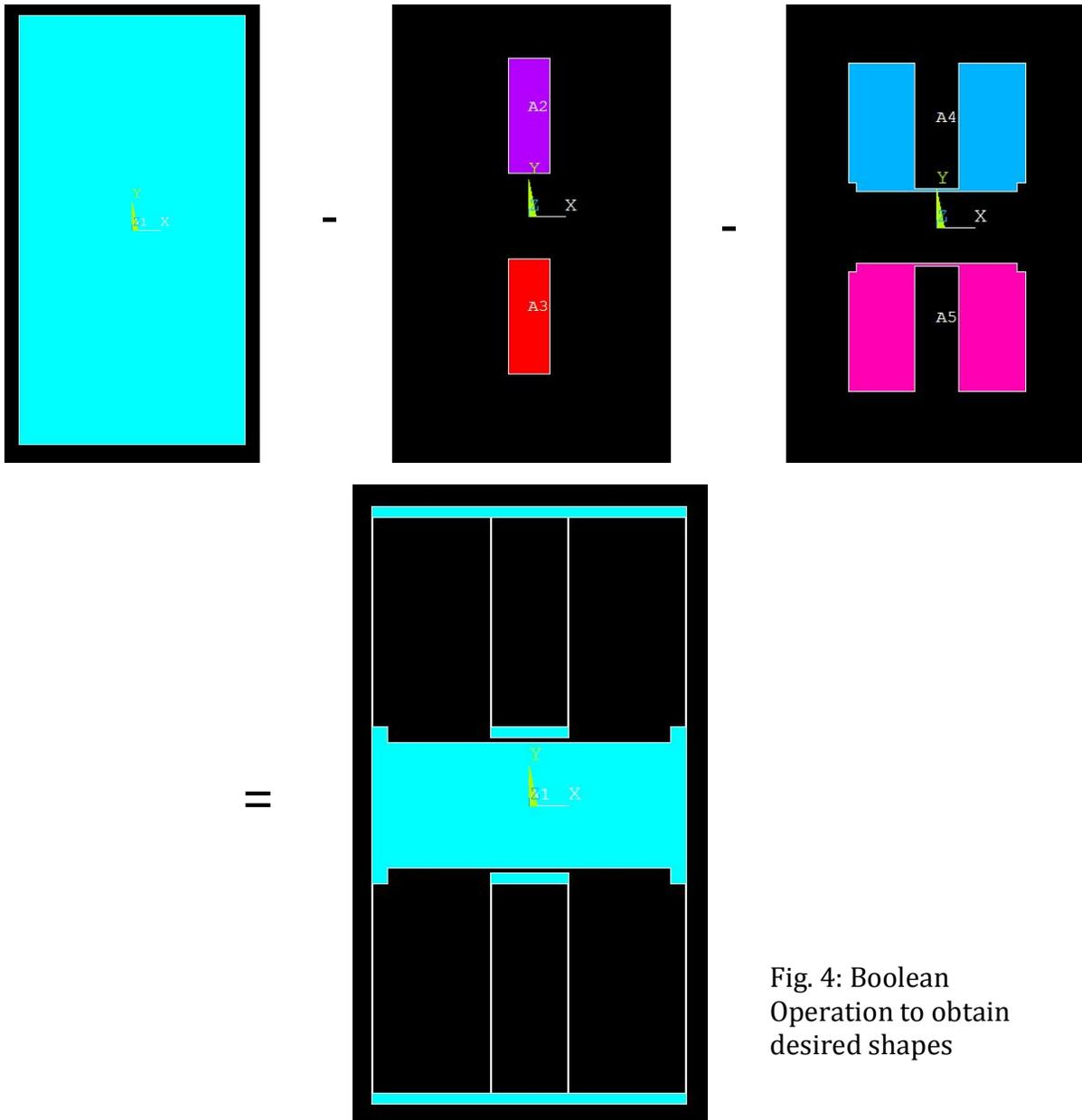
Fig. 4: Boolean Operation to obtain desired shapes
