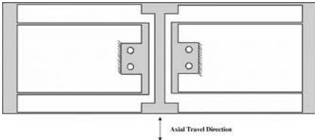
Figure 1. Folded Beam Suspension
